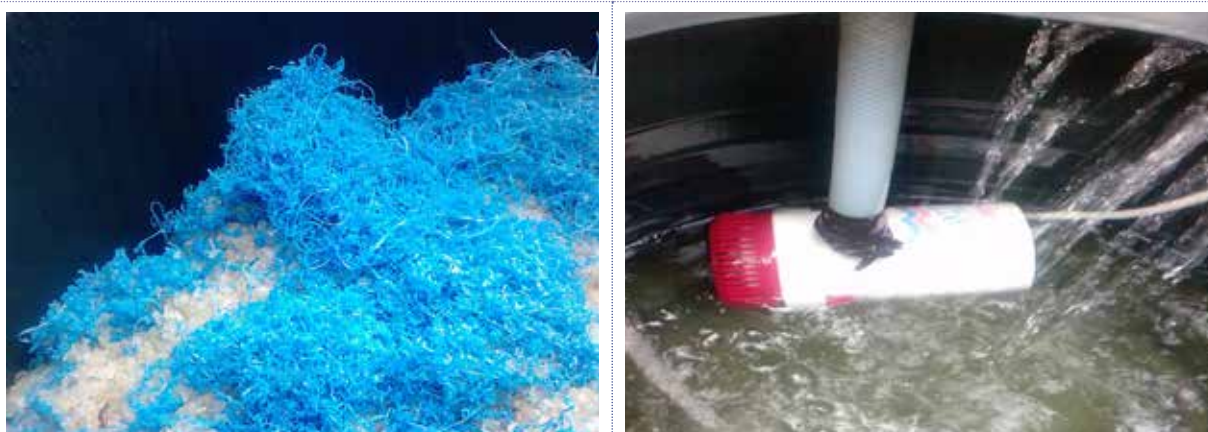
(a) Substrate used in biofilter. Plastic shaving or bottle tops (b) Submersible Pumps. Normally placed inside unit with filtered water
