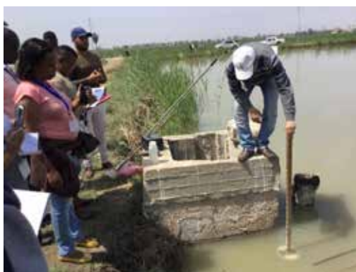
Figure 54: How to take Secchi Readings
